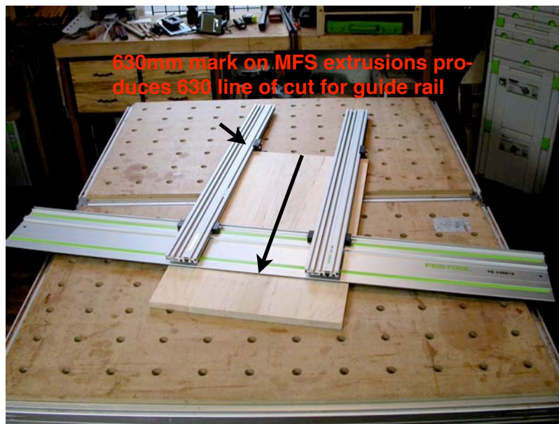
MFS extrusions with shop made saddles and stops set to position the guide rail for a 630mm cut
