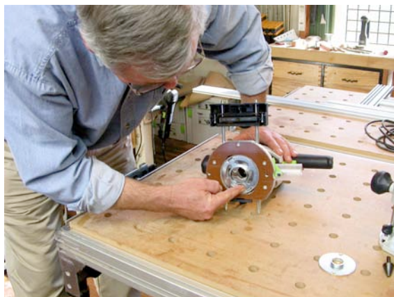
Guide bushings simply snap in place properly centered on 1400
