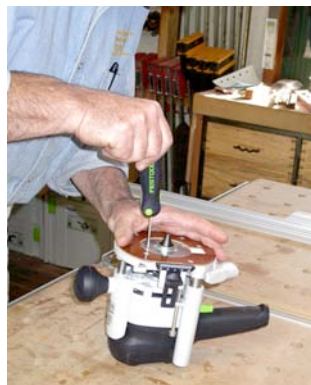
Guide bushing centered over mandrel and tightened down on 1010
