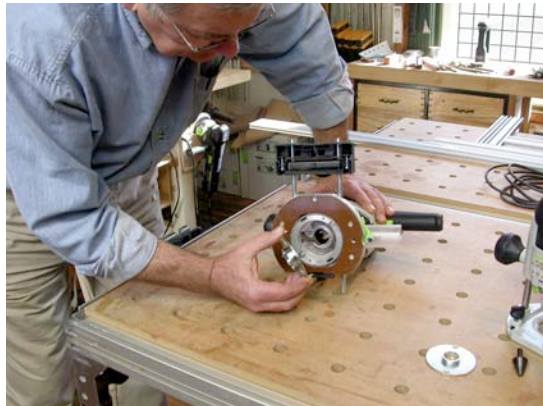
Guide bushings simply snap in place properly centered on 1400
