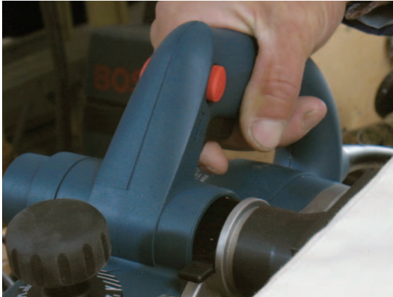
Figure 2. The safety lockout button on the Bosch planer (left) is in front of the trigger, so you have to either use two hands to start the tool or switch hand positions after starting it. The Festool’s safety switch is near the trigger (right). The Porter-Cable has no safety lockout.
