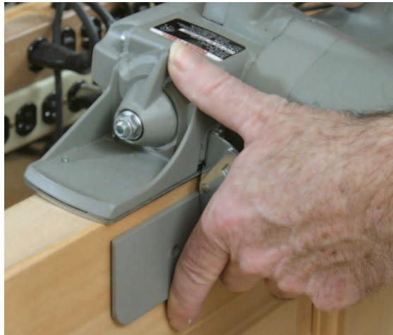
Figure 3. The fence on the Porter-Cable (left) cannot be removed, meaning this tool can be used only for planing the edges of doors or lumber. The Festool’s fence (below) is not only fully adjustable, but it can be taken off for surface planing.
